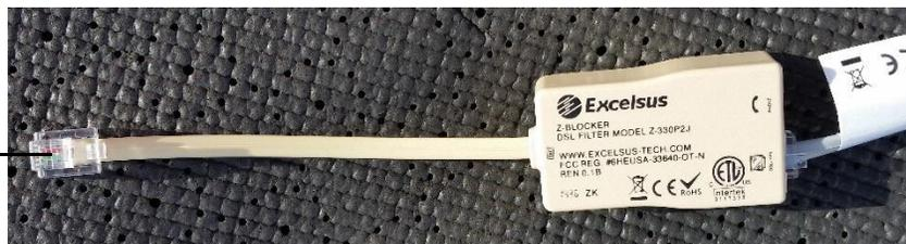
8. Plug a phone cord into the grey DSL filter port labeled “DSL/HPN”. Plug the other end of the phone cord into the grey port on the modem labeled “DSL”
